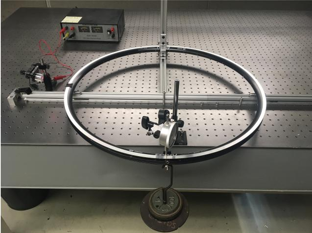
**Fig. 3** Four-point bending test. A small mirror resting on the rim at 9-o'clock reflects the laser spot onto a grid (to the right, not shown). The un-balanced configuration effectively doubles the lateral displacement at the load point and increases sensitivity.
